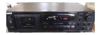
New belts (cost 12 pounds) just fitted, heads demagnetised and cleaned, capstan motor and flywheel relubricated. The deck is in good working order and cosmetic condition. See photo of the review in the October 1991 issue of Hi-Fi Choice where it won a Recommended Award. Dolby B/C, HX Pro, 3 motors, 3 heads (for off-tape monitoring) and manual bias adjustment are just a few of the features. Happy to.
