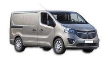
Engine size: 1.6 litre, Body type: Crew Bus, Fuel type: Diesel, Fuel delivery: Turbo, Transmission type: Manual, Drivetrain: Front Wheel Drive, Number of Seats: 6, CO2 Emissions: 160 g/km, Top Speed: 107 mph, Fuel Economy Combined: 46.3 mpg, Brake Horse Power: 120 bhp, Warranty years: 1 years, Warranty mileage: Unlimited, 0-62 mph: 13 secs, Manufacturer RRP: £27688.00, P11D: £27448.00, Benefit in kind (BIK): £8783.00, BIK @ 20% tax: £146.38 pcm, BIK @ 40% tax: £292.77
