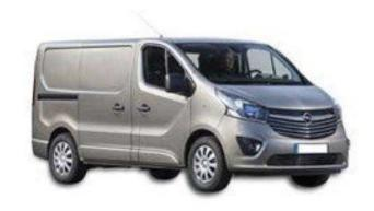
Engine size: 1.6 litre, Body type: Van, Fuel type: Diesel, Fuel delivery: Turbo, Transmission type: Manual, Drivetrain: Front Wheel Drive, Number of Seats: 3, CO2 Emissions: 155 g/km, Top Speed: 107 mph, Fuel Economy Combined: 47.9 mpg, Brake Horse Power: 120 bhp, Warranty years: 1 years, Warranty mileage: Unlimited, 0-62 mph: 13 secs, Manufacturer RRP: £27328.00, P11D: £27088.00, Benefit in kind (BIK): £8397.00, BIK @ 20% tax: £139.95 pcm, BIK @ 40% tax: £279.90
