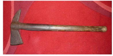
This XL axe measures 24.5" long x 9.5" across the head. It's the same style as a fireman's belt axe but far larger so was maybe kept on the vehicle to help break into buildings etc or used aboard trains for the same reason? The wooden shaft is solid with no.
