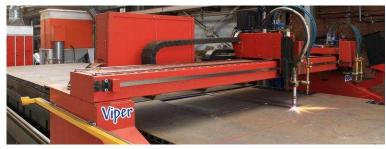
The CNC Oxy-fuel technology is still relevant in Metallurgy. For cutting metals whose thickness is more than 50 mm, the machinery is still used very much. Esprit Automation is showcasing before you a wide range of Oxy-fuel devices. A combined machine made with Oxy-fuel and Plasma by Esprit Automation can cut thick metals quickly. To get business opportunity visit espritautomation dot
