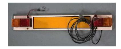
Light board with number plate for cycle/bike carrier or trailer. All in good working order with seven pin plug.
