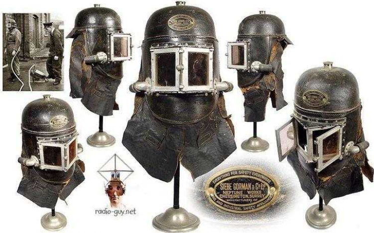
Siebe Gorman Mask circa 1878- Mfg'd by Siebe Gorman & Co. LTD, London England. Leather mask is attached to a hose, which is attached to a foot bellows. The firefighter would don the leather mask, while a second firefighter would provide air by operating a foot bellows. Signals were given by tugs on the hose by the wearer, 1 tug meant more air, 2 tugs less air, 3 tugs help me out.
